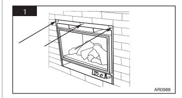
Place the backplate over the locating lugs and fully engage to ensure secure fixing.
